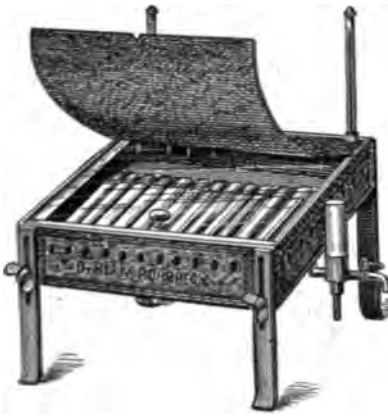
Fig. 5.—Inspissator. Koch's apparatus for coagulating and sterilizing blood-serum (McFarland).
